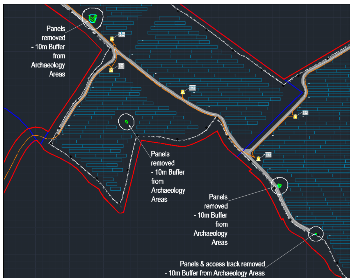
Figure 12: Archaeological features identified in Kilcommock Glebe (Trenches 41, 53, 61 and 62) buffered in solar farm design, access track remains within 10m of two features, to be monitored
